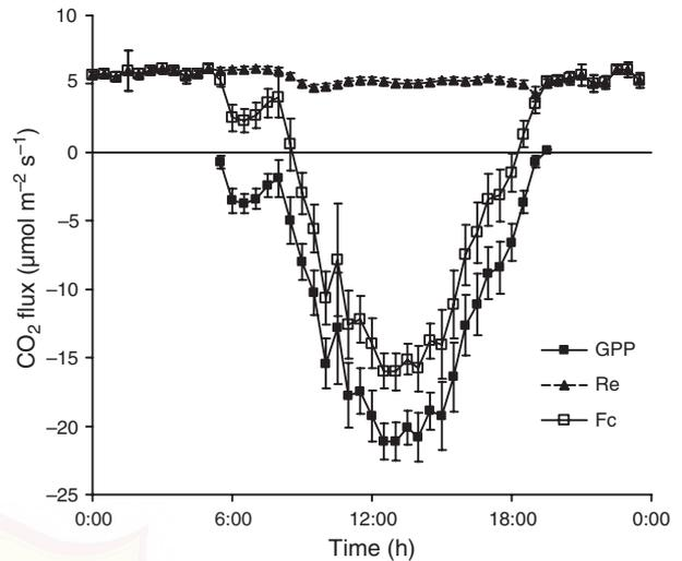
**Fig. 6.** Component fluxes ( $F_c$ ,  $R_e$ ,  $GPP$ ) derived from eddy covariance data from the Howard Springs site during the early wet season 16–29 December 2001. Data are 13-day ensemble averages, with error bars the standard error of the mean.
