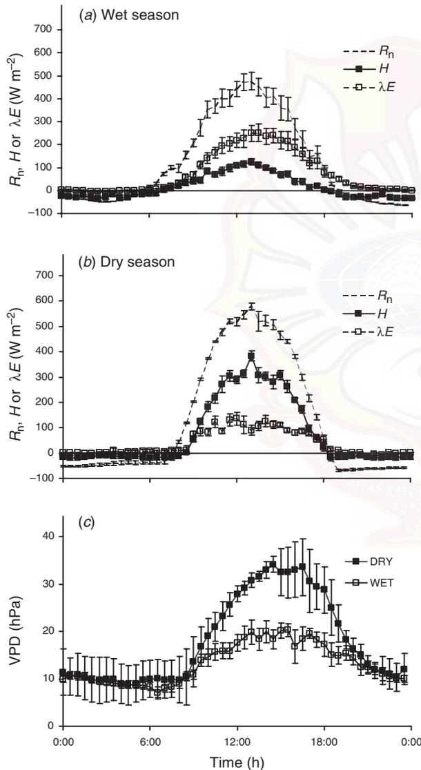
**Fig. 2.** Typical diurnal variation in 30-min fluxes of (a, b) sensible ( $H$ ) and latent heat ( $\lambda E$ ) and net radiation ( $R_n$ ), and (c) vapour pressure deficit ( $VPD$ ) at the Howard Springs eddy covariance site. Data are shown for (a) the dry season, August 2001, and (b) the following wet season, February 2002. Data are 7-day ensemble averages, with error bars the standard error of the mean.
